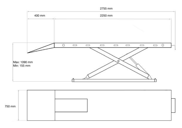
Hospital Bed Maintenance Lift platform dimensions with the WEK (width extension kit).
